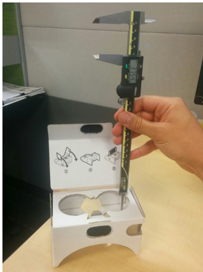
Figure 16. Distance between the back surface to screen (distance D in table 13).
